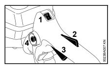
The stop switch (1) is in the normal run position I.
