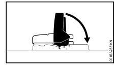
Fold the grip down so that it is flush with the top of the cap.
