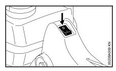
Move the stop switch in the direction of 0 – when released, the stop switch springs back to the normal run position I.
