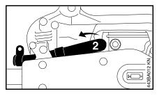
Remove the exhaust pipe (2).
