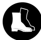
Wear **safety boots** with steel toe caps and non-slip soles.
